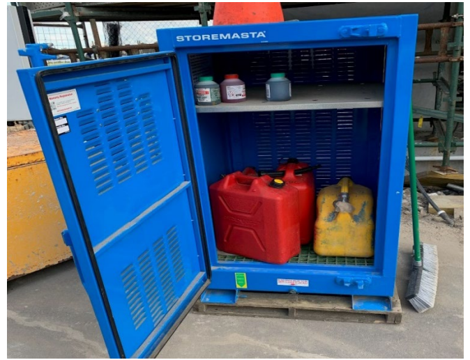
Photo 6: Fuel Storage Cabinet
